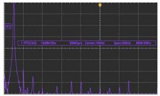
1kHz/1V sine wave input tone (left peak) with the resulting multi frequency harmonics peaks in purple.
